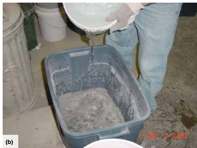
Fig. 1: Preparation of the base layer in a 16 x 29 x 15 in. test container: (a) compacting the 4 in. base layer; and (b) adding 16 lb of an \text{Na}_2\text{SO}_4 solution to the base layer
