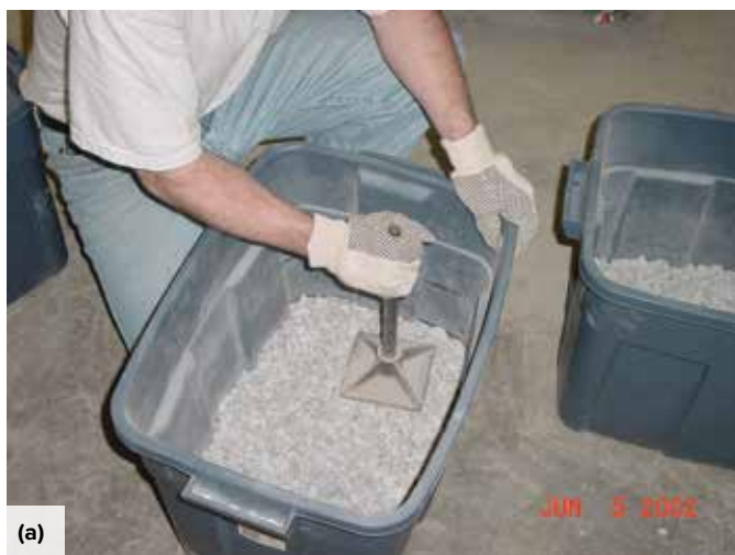
Fig. 1: Preparation of the base layer in a 16 x 29 x 15 in. test container: (a) compacting the 4 in. base layer; and (b) adding 16 lb of an \text{Na}_2\text{SO}_4 solution to the base layer
