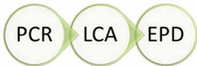
Fig. 2: The sequence of processing an EPD. Product category rules (PCRs) define parameters for a life-cycle analysis (LCA) used to generate an EPD (courtesy of Long Trail Sustainability website)
