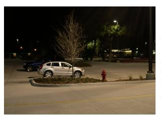
Further calculations showed that comparable luminance could also be achieved on the concrete parking lot with a reduction in illuminance. In fact, if the wattage in each of the 22 luminaires on the concrete lot was reduced from 400 W to 250 W, the average luminance of .336 cd/ft<sup>2</sup> was still greater
