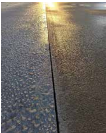
Wet concrete surface with (left) and without (right) a penetrating sealer
